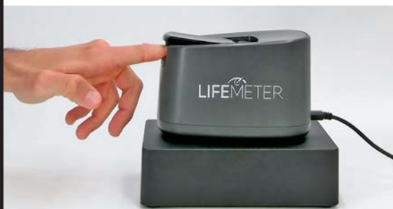
The LifeMeter device being used to measure a patient's carotenoid levels. The patient just puts a forefinger into the LifeMeter measuring instrument.
